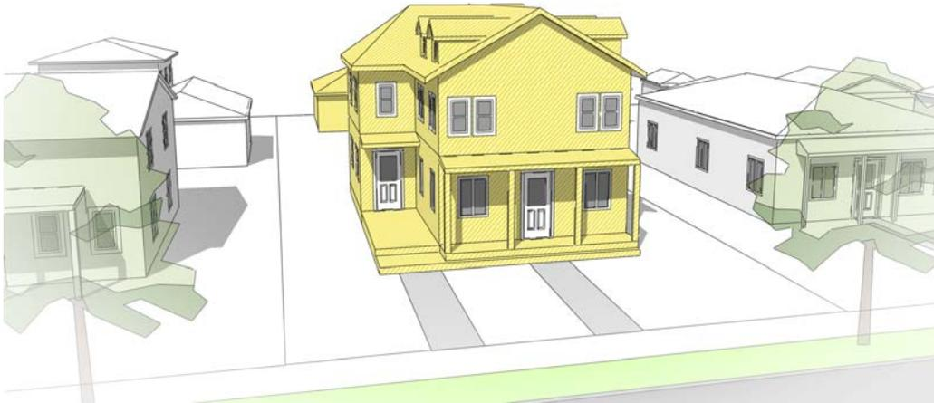
**Figure 6—Use of offset and variation in building massing to distinguish between entrances in street-facing duplex units.**
